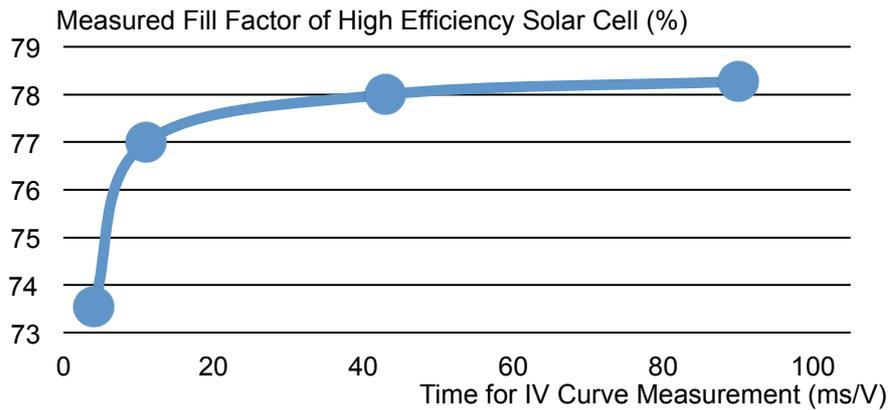
Figure 2: Measured fill factor of a single high efficiency solar cell for different voltage sweep times. The measurement shows that this specific high efficiency solar cells needs a minimum sweep time of 80 ms/V.
