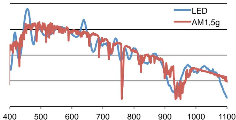
Figure 1: Comparison of the sun's spectrum with the spectrum achievable with state-of-the-art LEDs. The deviation from the target values for the ranges 400-500nm, 500-600nm, ... is below 1%.
